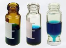
NOT ALL GLASS VIALS ARE CREATED EQUAL AND THEY ARE NOT INERT. The glass surface is covered with highly reactive silanols that can interact with your samples by changing pH, hydrolyzing or adsorbing it and lowering your quantitation results with a poor RSD.
